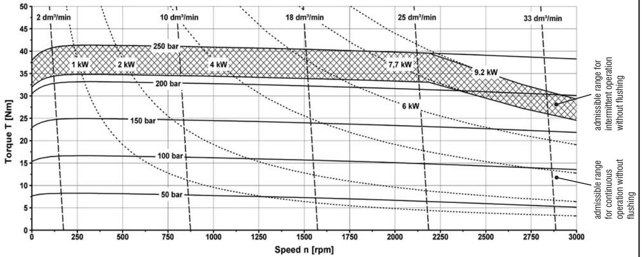
hydraulic and mechanical efficiency by %
