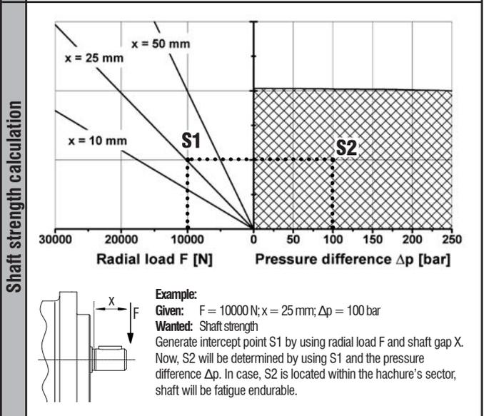
All parameters at  $v = 32 \text{ mm}^2/\text{s}$ ;  $\Theta = 40^\circ\text{C}$ ;  $p_{\text{outlet}} = \text{pressureless}$
